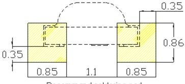
Recommand soldering pad
