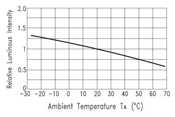
Fig.5 Luminous Intensity vs.Ambient Temperature
