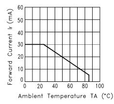
Fig.3 FORWARD CURRENT DERATING CURVE
